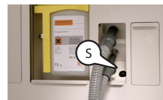
Suction hoses fitted at disinfection nipples.
