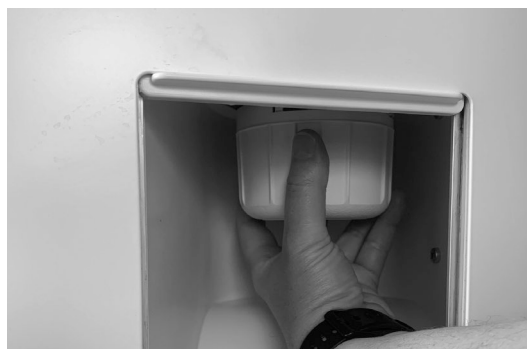
Figure 76 – Replacing the amalgam collector vessel.
