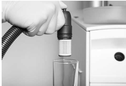
Figure 72 – Press the button to eject the filter holder and cartridge.
