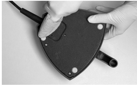
Figure 15 – Degreasing of foot control's "rubber feet".
