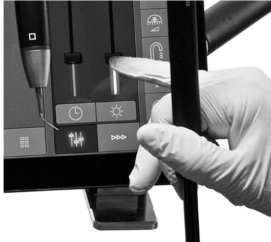
Figure 17 – Use the little finger of the hand holding the instrument to control buttons and sliders in the instrument control window.
