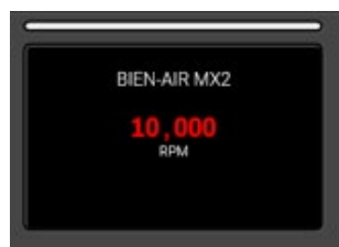
Figure 19 – Instrument display when a micromotor is activated showing actual speed.
