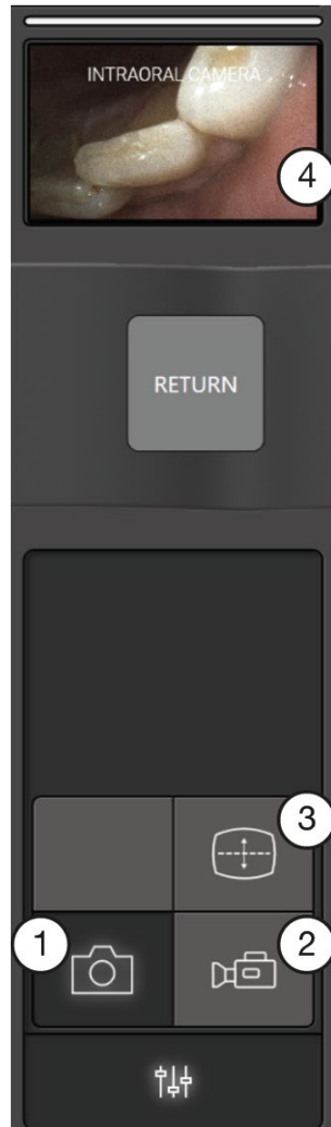
Figure 36 – Instrument control window and display for intraoral camera: (1) camera mode, (2) video mode, (3) rotate image 180°, (4) live image.
