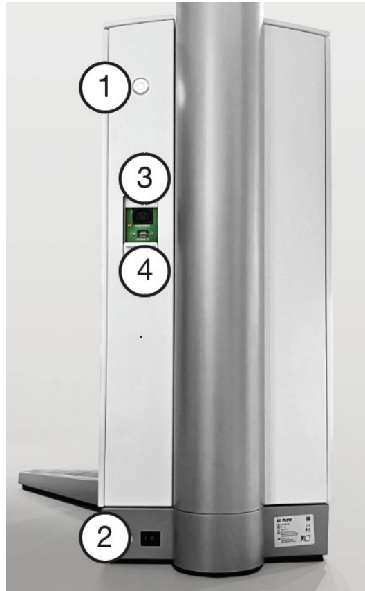
Figure 2 – Rear panel: (1) on switch, (2) mains switch, (3) 230 V socket, (4) external USB port.
