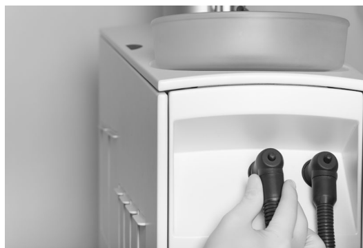
Figure 71 – Removal of suction filters.
