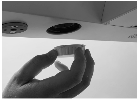
Figure 64 – Accessing the oil separator sponge.
