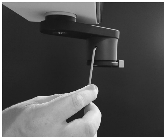
Figure 43 – Adjusting the tray holder mechanism rotational friction brake
