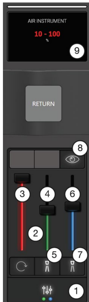
Figure 22 – Instrument control window and display for an air instrument: (1) button (incl. spray water and air indicators) for opening and closing instrument control window, (2) instrument control window, (3) drive air range slider, (4) spray water slider, (5) spray water on/off button, (6) spray air slider, (7) spray air on/off button, (8) automatic chip blow on/off button, (9) instrument display.
