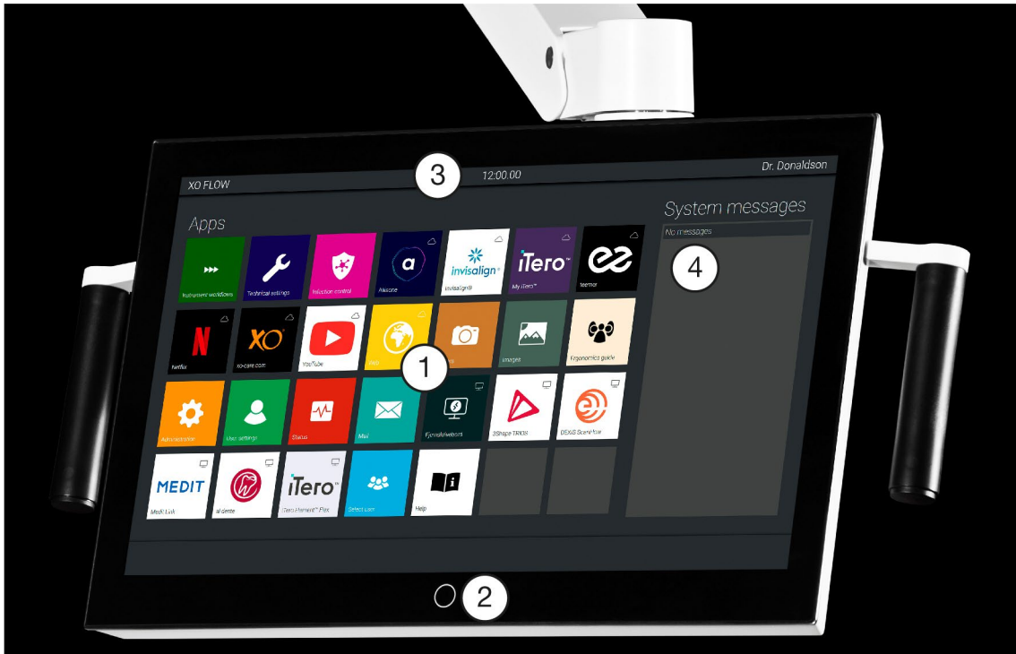
Figure 5 – Navigator home screen: (1) XO dental apps, (2) home button, (3) information bar, (4) system message window.
