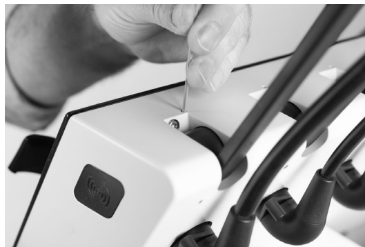
Figure 13 – Adjustment of instrument suspension angle.
